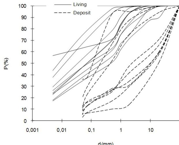
Fig. 3. Particle distributions of weak coherent debris flows.
