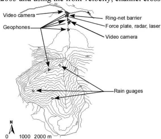
Fig. 1. Instruments location of at the Illgraben test site.
